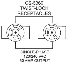
Figure 10. 120/240V Twist-Lock Auxiliary Receptacles Each auxilliary receptacle is protected by a 50 amp circuit breaker. These breakers are located directly above the GFCI receptacles. Remember the load output (current) on all three receptacles is dependent on the load requirements of the *Output Terminal Lugs*.
